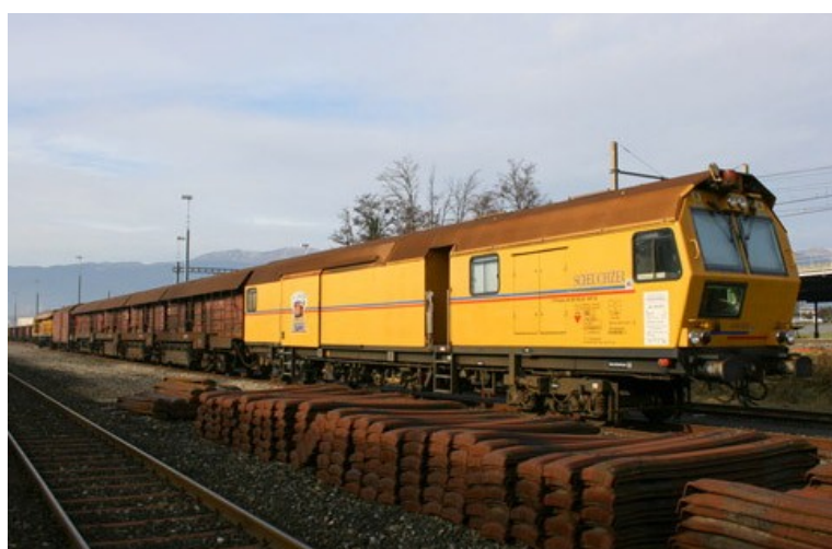
Figure 15: Train meuleur de rails (Scheuchzer S.A.)
